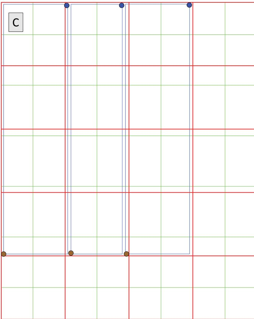
This is how the graph paper shown left should be used for a 3 x 4 metre room layout. The eyelet positions have been included as has the location of the controller. In this instance two 1000mm wide mats and one 800mm mat have been used. Total power consumption for this arrangement would be about 2460 watts. The illustration below is drawn from the graph.
