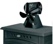
The device works on a simple principle; the hotter the bottom and the colder the top, the more electricity is generated. By utilising a fan on the top section and by incorporating an aerodynamically designed front fan blade, the SmartFan can move air up to a rate of 360 Cubic Meter per hour (200 Cubic Feet per minute).
