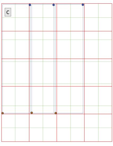
This is how the graph paper shown left should be used for a  $3 \times 4$  metre room layout. The eyelet positions have been included as has the location of the controller. In this instance two 1000mm wide mats and one 800mm mat have been used. Total power consumption for this arrangement would be about 2460 watts. The illustration below is drawn from the graph.
