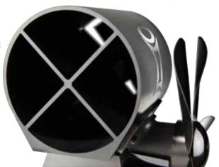
The SmartFan is a self-powered, clean, silent and efficient device that greatly improves heat circulation from your solid fuel burning stove. The device is powered by a thermoelectric generation module (TEM) which uses the hot surface of the stove to generate an electric current to propel two fan blades. Heat, instead of rising immediately to the ceiling, is propelled directly into the living space and provides an increased level of comfort and greater fuel efficiency.
